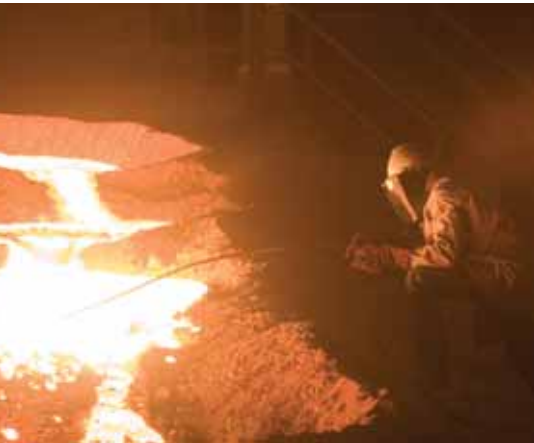
Boshoek Smelter, tapping of furnace
