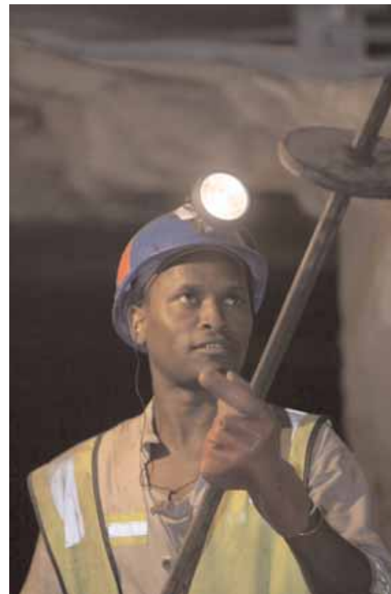
Franz Mazivhe 'sounds' the roof to check for roof fall hazards at Kroondal mine
