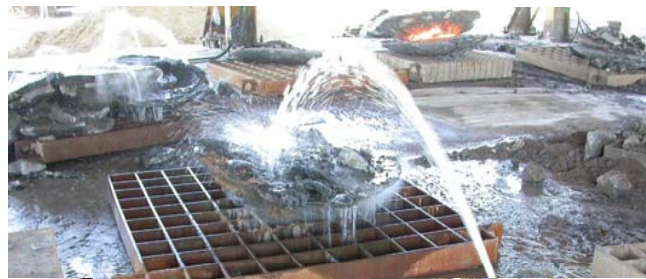
Extracted ingots undergoing final cooling before breaking
