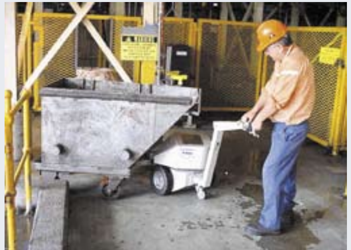
John Beldan, Machinery Operator Xstrata Copper, Townsville Refinery, manoeuvring a tramp copper bin with the Electrodrive battery tug.
