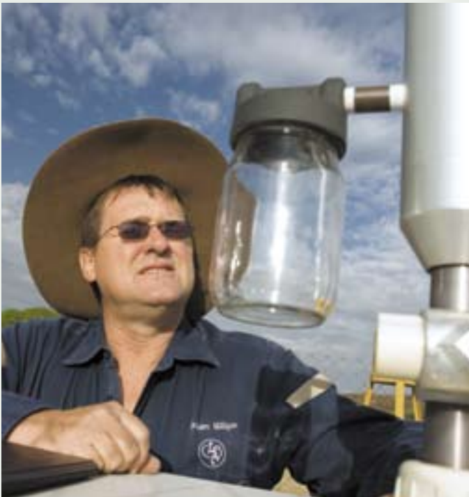
Graham Milligan, Environmental Sampler undertaking particulate (dust) monitoring at one of several monitoring stations located in the Mount Isa community.
