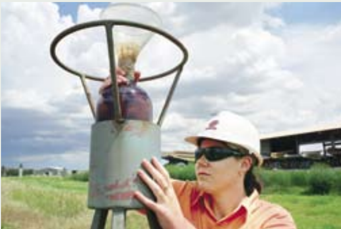
Raelene Green checks one of the dust monitoring points. There has been no identified increase in dust deposition or elevation copper concentration rates outside the Ernest Henry mine's term lease areas.
