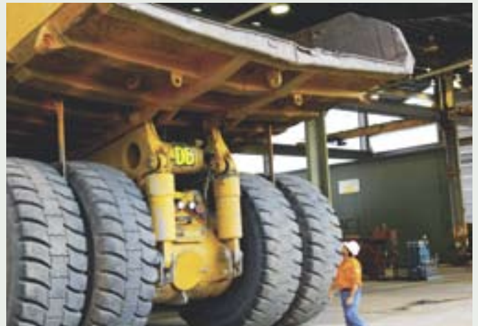
Pre-start check over all heavy equipment is part of daily operations: attention is paid to tyre condition.
