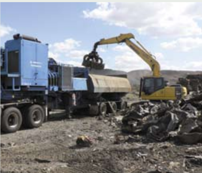
Light gauge scrap metal being compacted into bales for recycling off-site.
