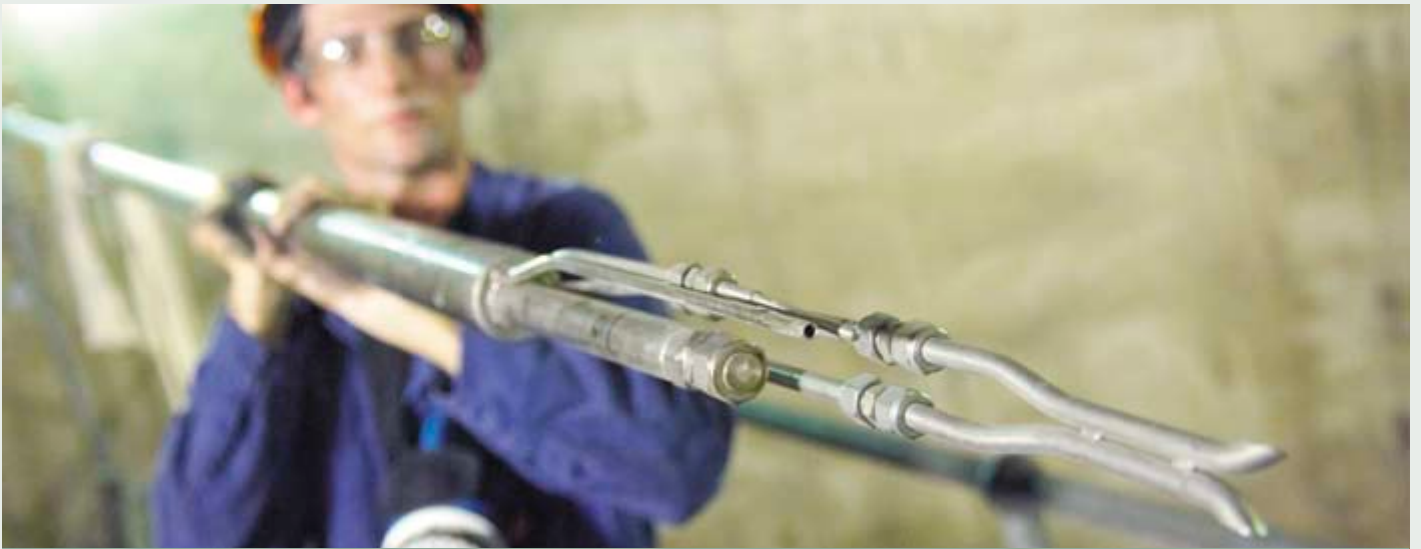
Xstrata Zinc employee, Matt Ashkar, takes a sample of production off-gases from the lead smelter stack.
