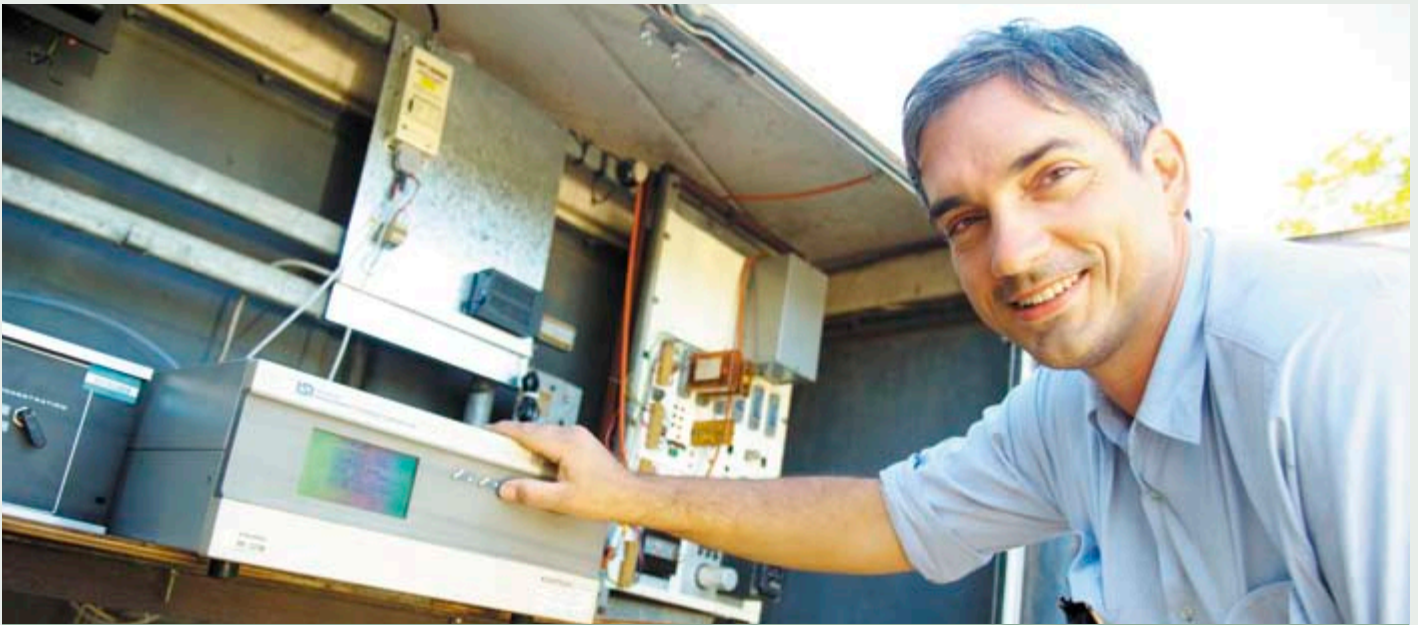
Electronics Technician, Marc Katona, conducts an instrument maintenance check of the sulphur dioxide monitors located in the Mount Isa community.
