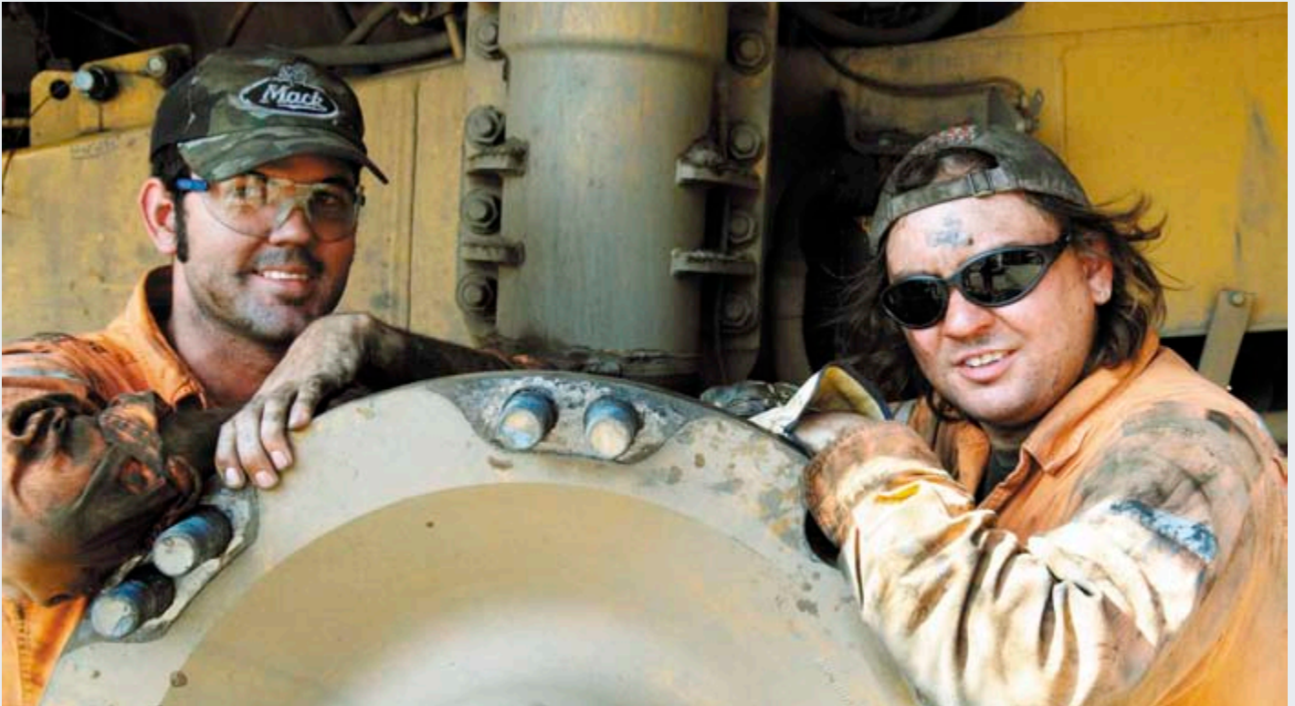
Adult Apprentice Diesel Fitter, Adam Briskey, and Diesel Fitter, Justin Preece, change brake calipers on a Caterpillar dump truck at the rebuild workshop at Mount Isa Mines. As part of our apprentice program, Xstrata encourages employees to consider a trade career and has an annual intake of adult apprentices from our existing workforce.
