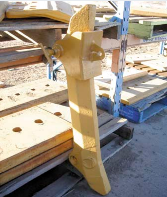
The goanna bar jig, an innovation from Ernest Henry mine to prevent manual handling of heavy dozer blade protectors.
