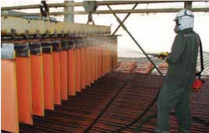
SX/EW plant operator, Juan Vargas Castro, washing copper cathodes at Xstrata Copper's Lomas Bayas operation in Chile
