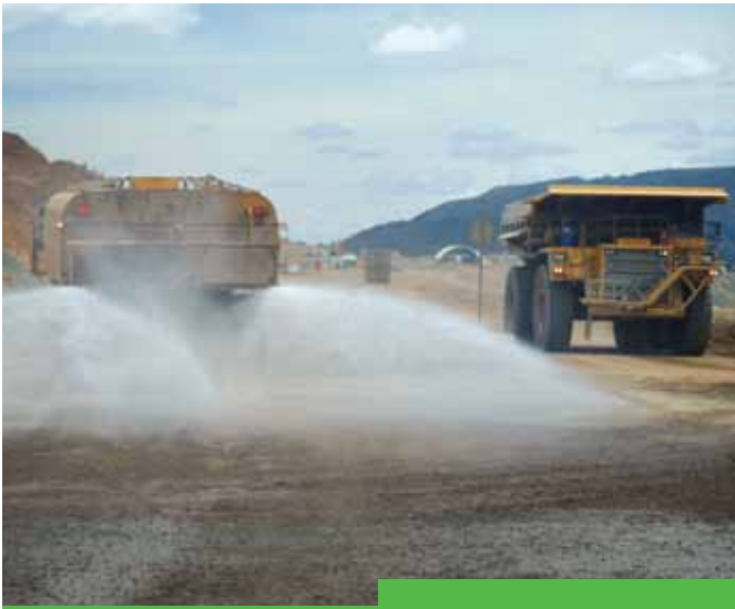
Water trucks are an integral part of dust suppression techniques used in Mount Isa operations.
